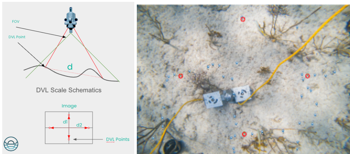
Figure 2. Schematic representation of Advanced Navigations Hydrus DVL scaling
