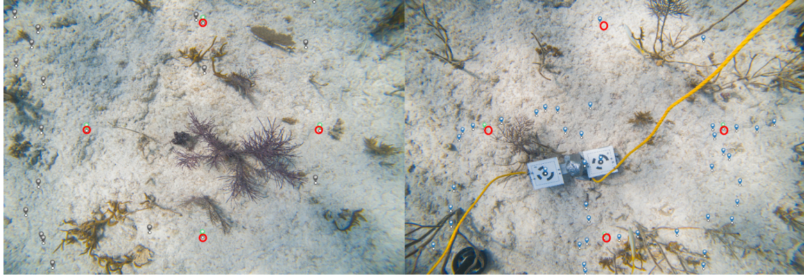
Figure 4. Images showing the DVL bounce positions (red circles) as markers in Metashape
